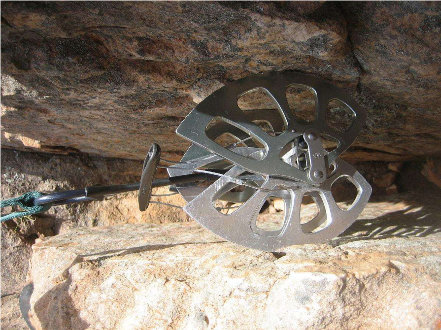
Figure 2 – Cam Engaged in a Crack
