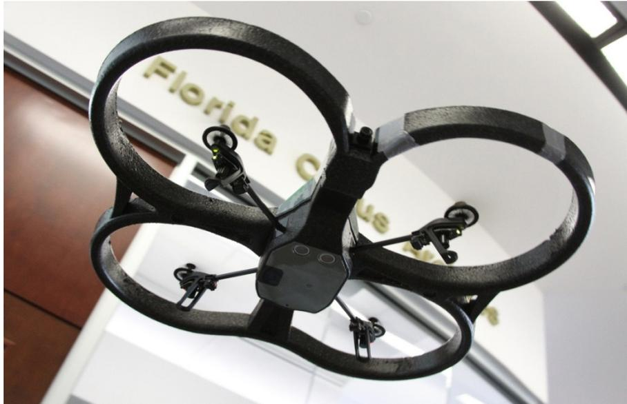
the front camera captures images at 720p, the streamed framerate is approximately 30 frames per second. Communication is via a Wi-Fi access point created by the vehicle. The API provided by Parrot supports a C++ interface allowing direct control of roll, pitch, yaw and thrust, making possible complete control of the vehicle via software.
